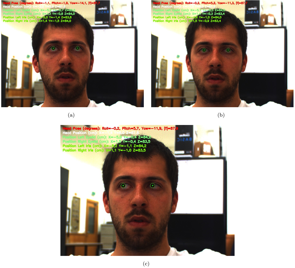
FIGURE 5.23: Three examples of the extraction of the 3D position of both irises, based on the (x, y) pixel position of the irises and the 3D Z position of the eyelids.
