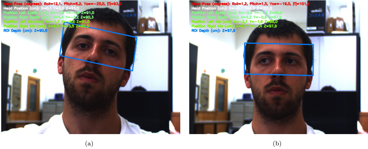
FIGURE 5.22: Examples of the eyes ROI, with different head poses (blue rectangle). The Z position of the ROI is shown in the left side of the image (blue text).
