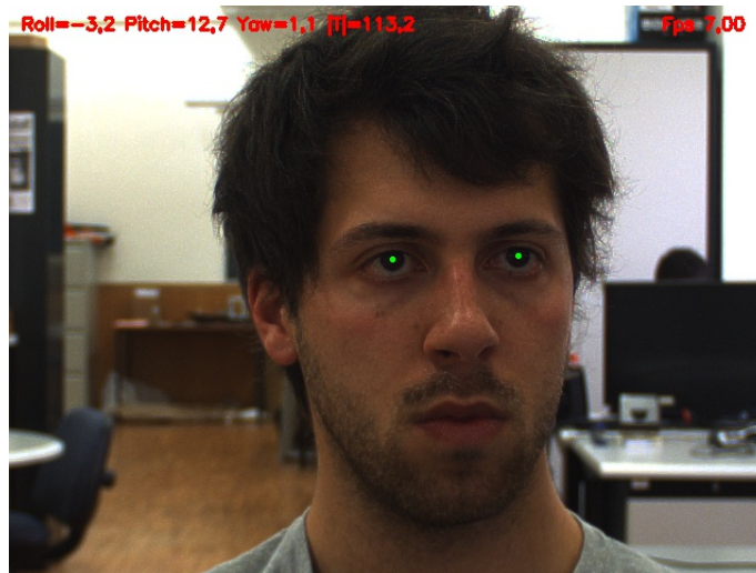
FIGURE 5.11: Detection of the iris center (green point) in a frame of a real time capture.
