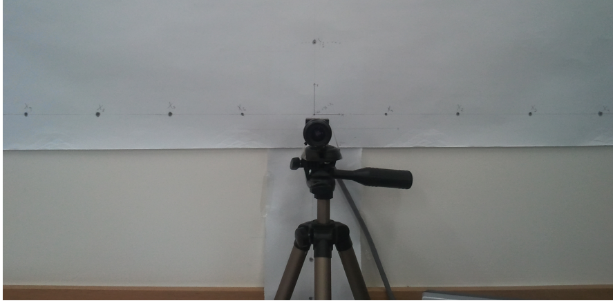
FIGURE 5.13: White board placed on the wall, parallel to the camera XY plane.
